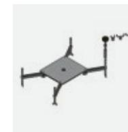
**Aggregate plate with supporting arms:** Particularly versatile aggregate plate for the removal and installation of engines, transmissions, axles, exhaust systems, etc. Extendable supporting arms with integrated threaded spindles and numerous support components allow easy adaptation to different mounting requirements (Art. No.: 103802)
