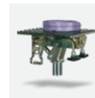
**GA passenger car:** Universally applicable for passenger cars. Particularly suitable for automatic transmissions. Tensioning strap to secure the load, large rubber supporting surface, load capacity 400 kg,  $\varnothing$  35 mm pin, dimensions 300 x 240 mm (Only applicable in combination with universal adapter, Art. No.: 103544) (Part No.: 3136)
